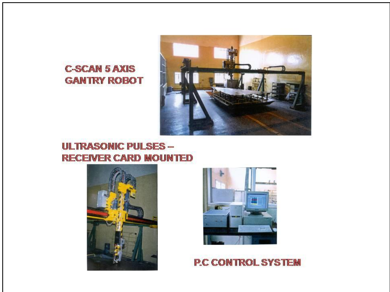
Fig. 3: C-SCAN 5 AXIS GANTRY ROBOT
